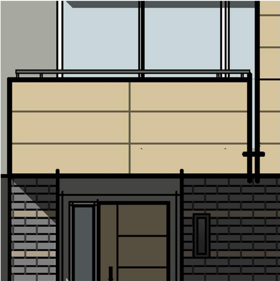
5 METAL RAILING METAL RAILING WITH PANEL SIDING
