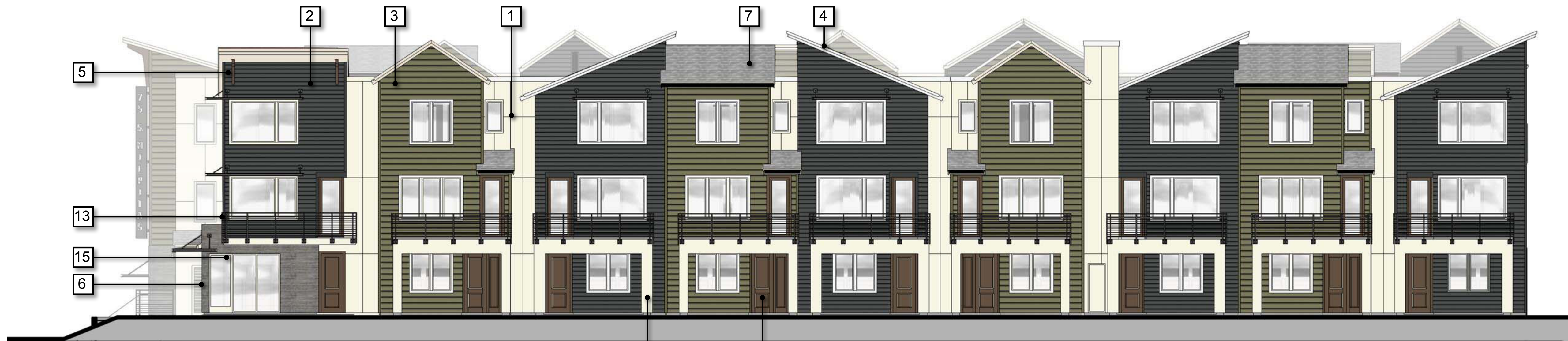
901 BUILDING - FRONT ELEVATION E SCALE: 1/8" = 1'-0"
