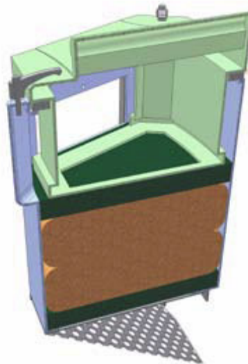
Figure 5: Cut-away view of the Filter Module
