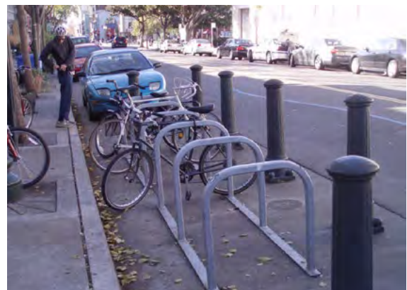
IN LOCATIONS WITH HIGHER DEMAND, BIKE CORRALS CAN CREATE MORE PARKING OPTIONS FOR BICYCLES. IF IMPLEMENTED ON STREET, AS SHOWN ABOVE, THEY ALSO CAN PROVIDE TRAFFIC CALMING AND ENHANCE THE PEDESTRIAN ENVIRONMENT.
