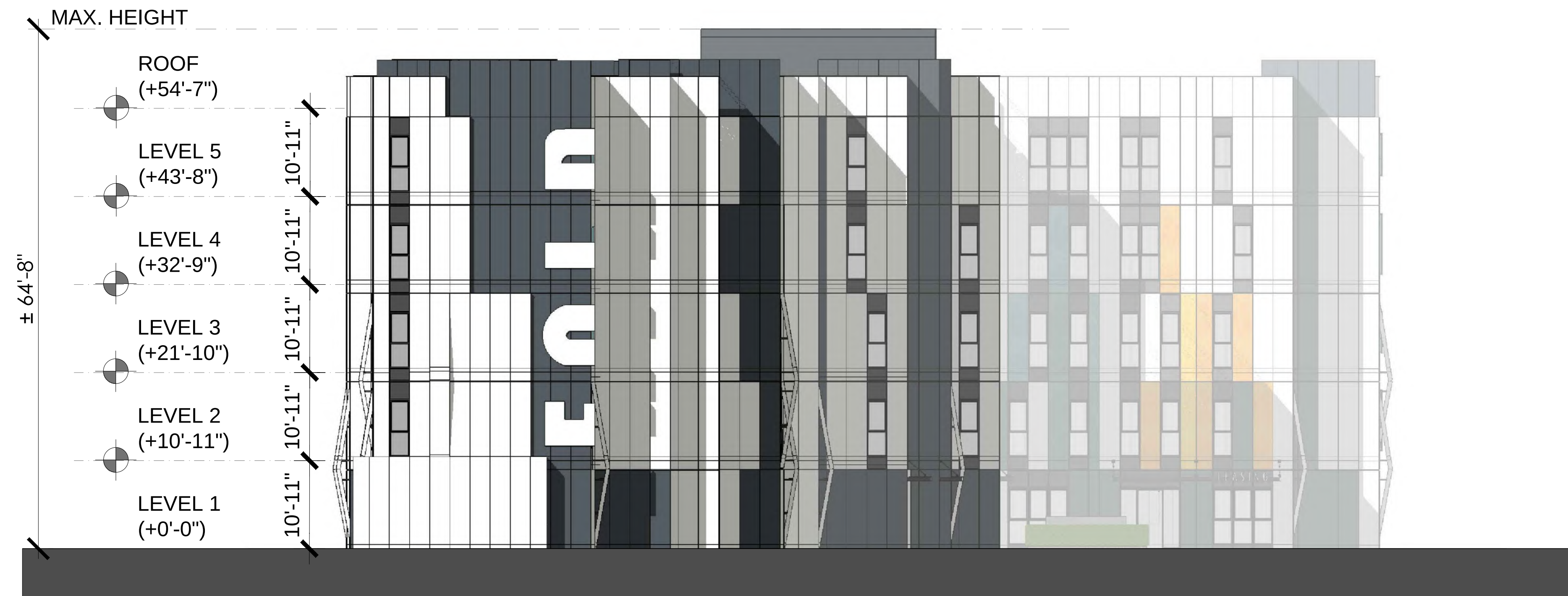
BUILDING A - NORTH ELEVATION 1
