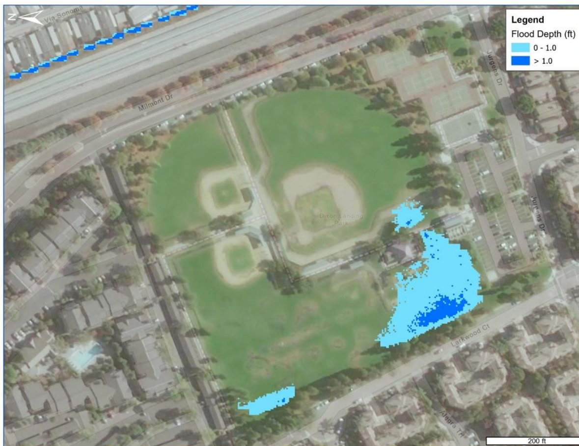
Figure 4-2: 10-year Ponding Adjacent to Jurgens Pump Station
