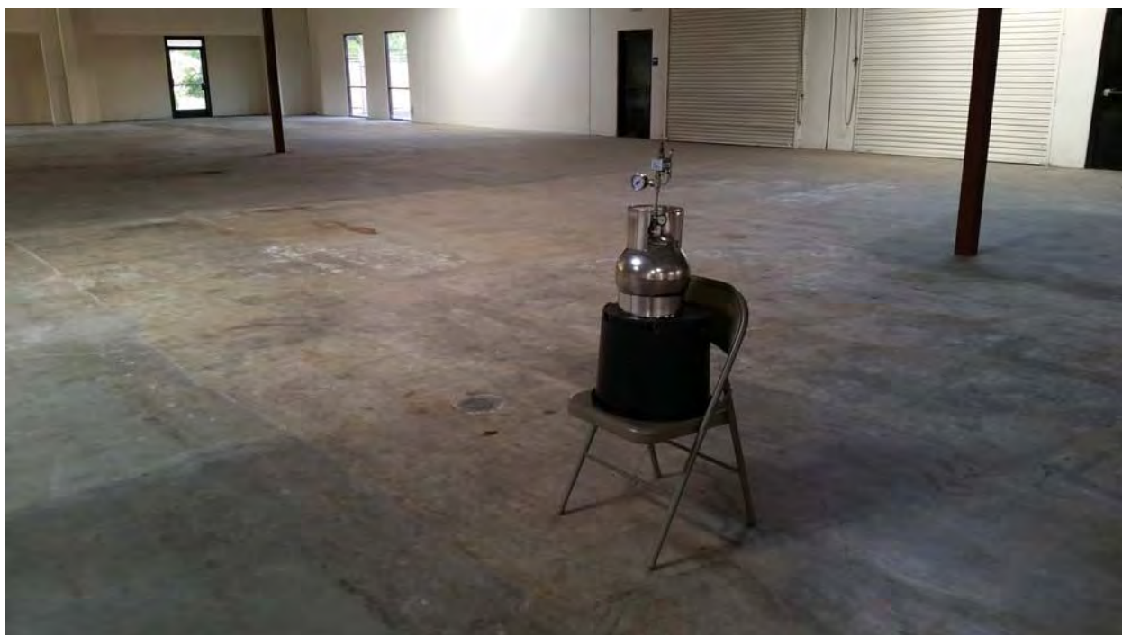
Indoor Air Sample Canister, Warehouse
