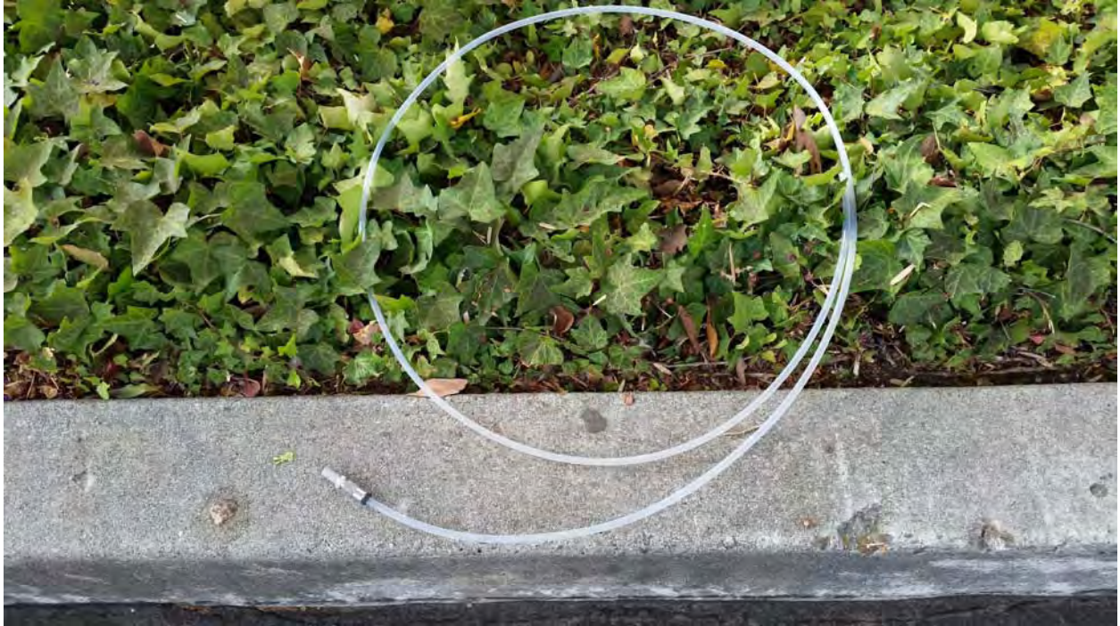
Soil Gas Probe
