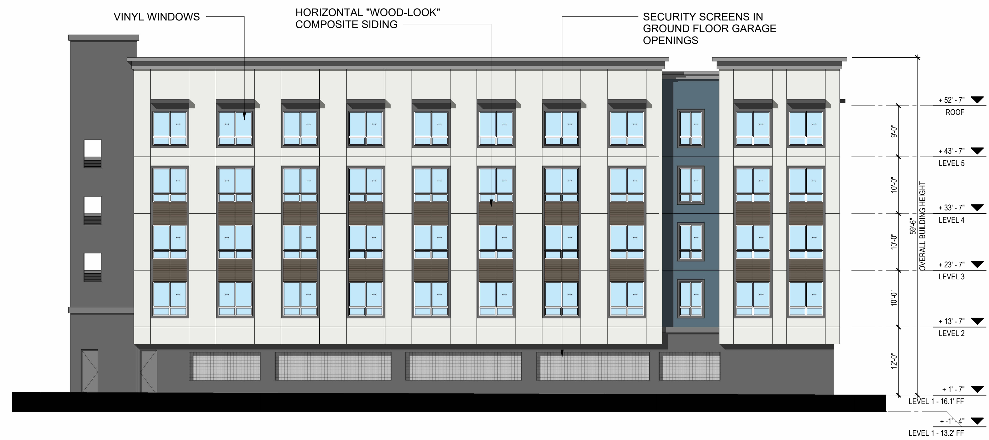
BLDG ELEVATION - WEST 3/32" = 1'-0" 2
