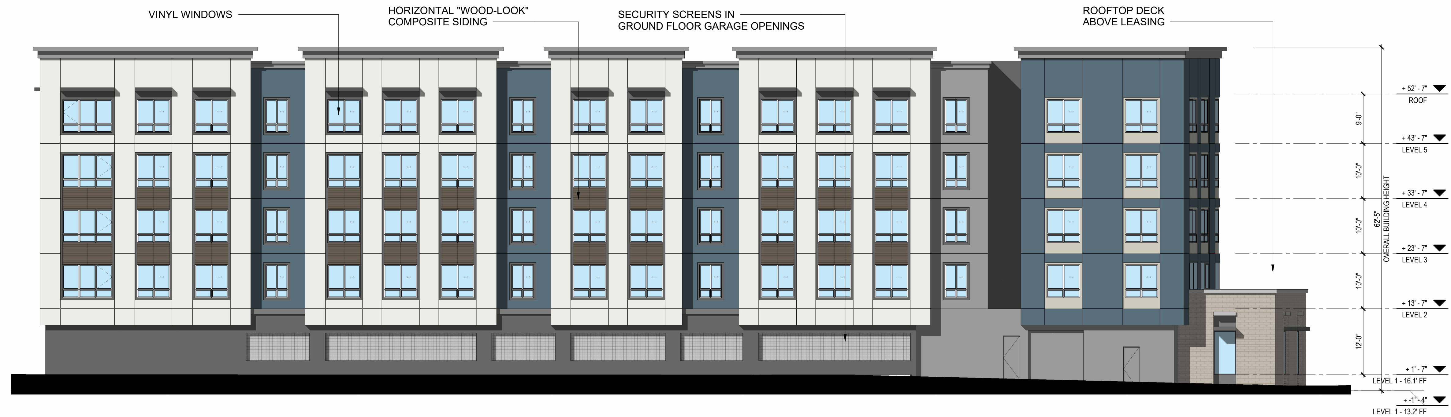
BLDG ELEVATION - SOUTH 3/32" = 1'-0" 2
