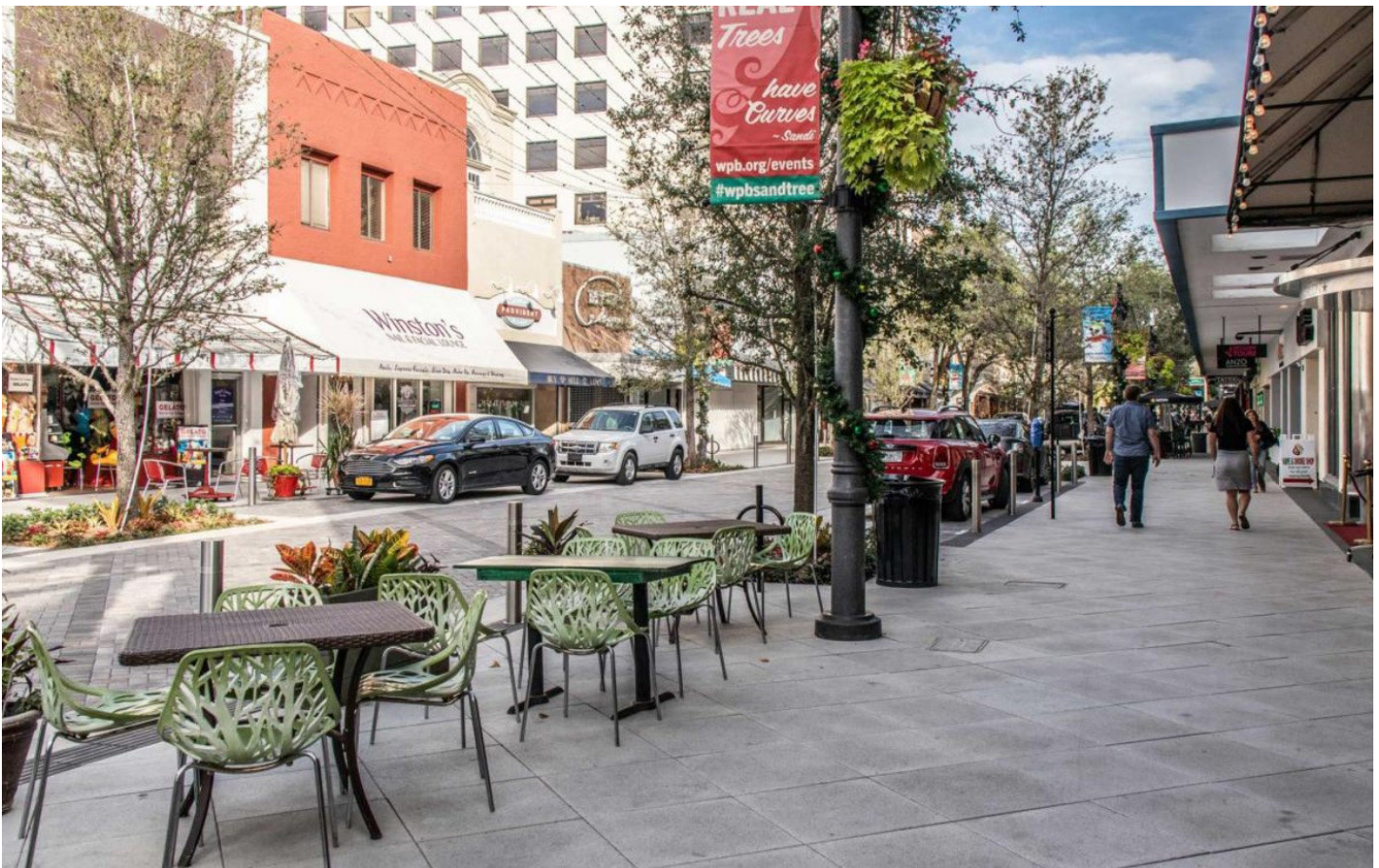
An example of a Shared Street with curbless right-of-way and varied pavers to distinguish between sidewalk and shared roadway.
