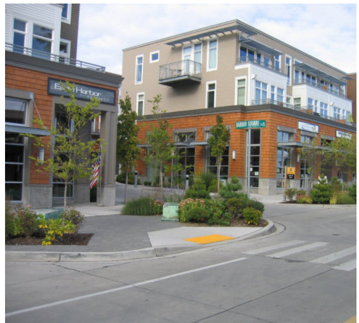
A planted curb extension at an intersection.
