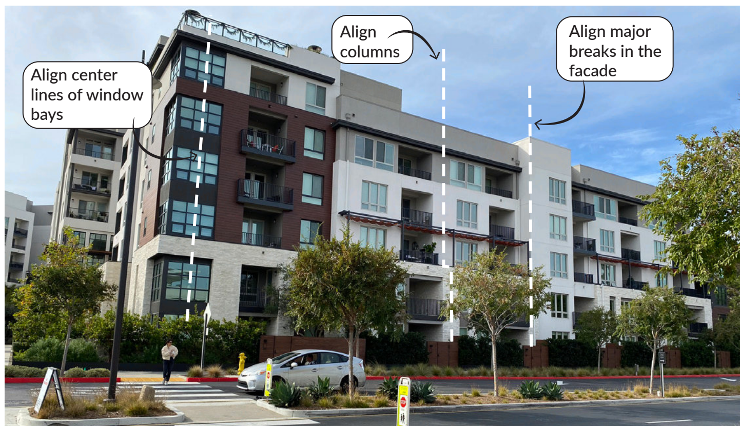
Figure 4-11 Upper Floor Alignment
